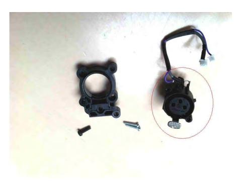
Separate the connector section from the XLR chassis
